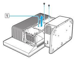
7 Unscrew the four screws on the drive holder (1).
